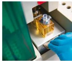
Analysis and sorting of a sample using flow cytometry on the ICV platform
